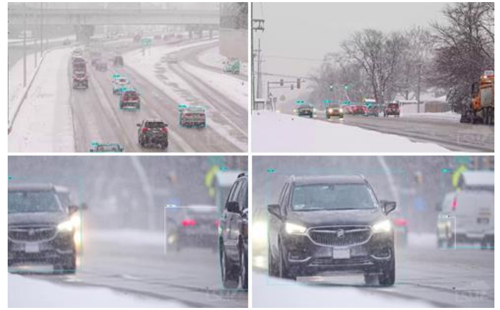
Figure 34. Detection of the Faster R-CNN in Snowy Weather Condition
