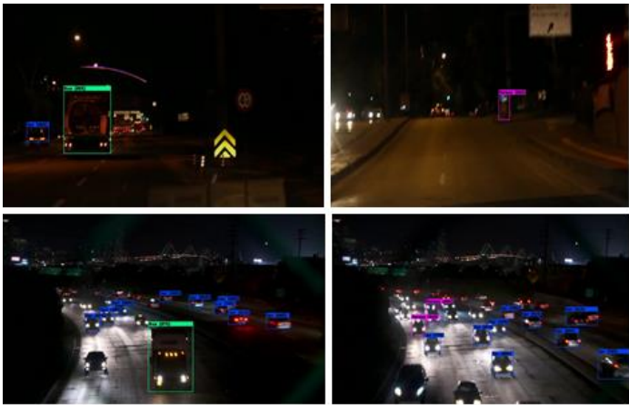
Figure 14. Wrong Detection and Errors of YOLOv4 at Night
