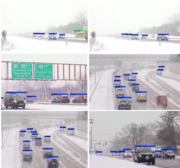
Figure 19. YOLOv4 Detection Result in Snow Weather
