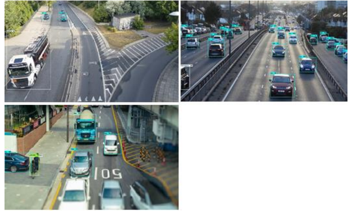
Figure 29. Wrong Detection for the Faster R-CNN at Daylight
