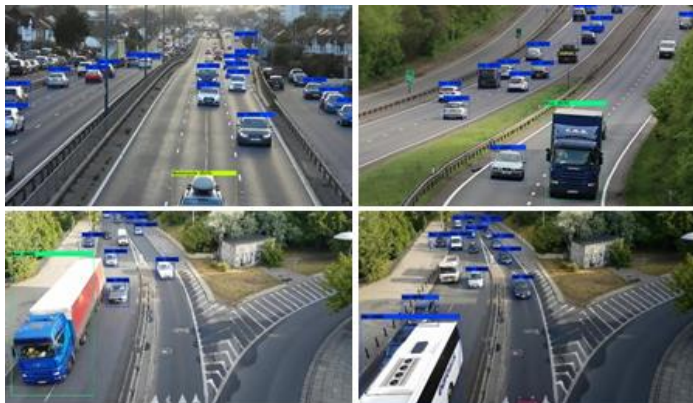
Figure 21. Wrong Detection of YOLOv3
