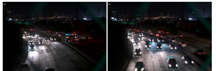
Figure 31. Wrong Detection of the Faster R-CNN at Night
