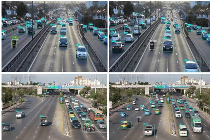
Figure 28. Detection of Faster R-CNN at Daylight
