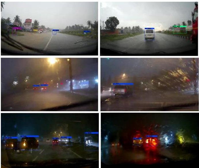
Figure 15. YOLOv4 Detection Results Under Heavy Rain Condition
