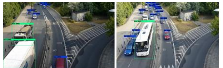
Figure 12. Wrong Detection of the Long-Track as a Bus With YOLOV4
