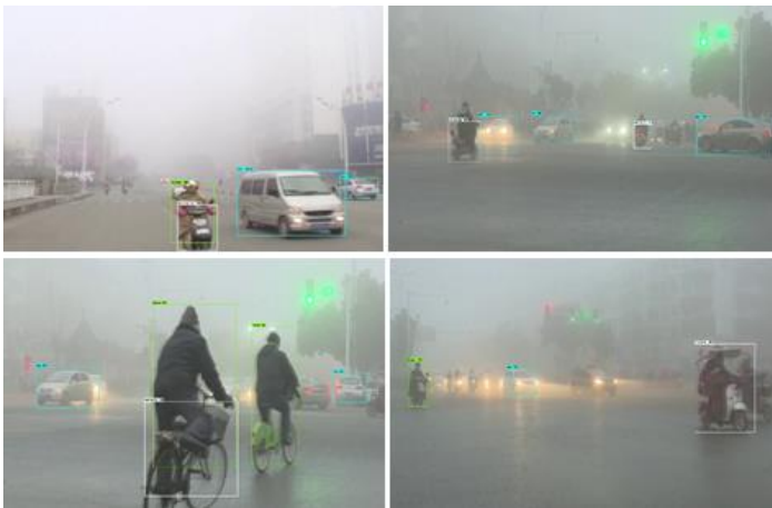
Figure 33. Detection of the Faster R-CNN in Foggy Weather Conditions
