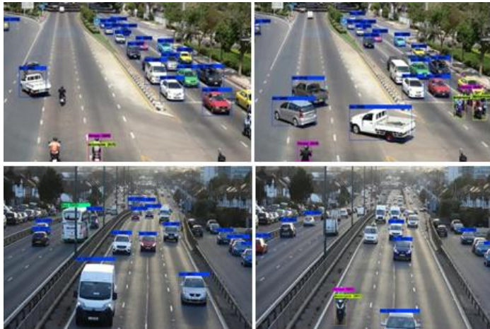
Figure 20. Detection for YOLOv3 at Daylight
