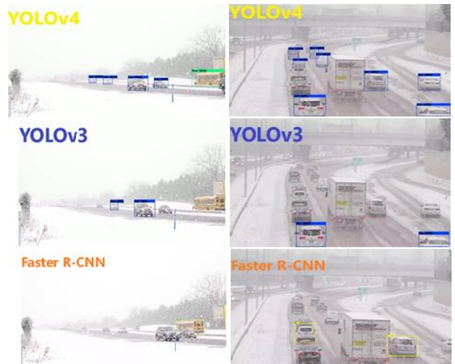
Figure 38. Detection of YOLO, and Faster R-CNN in Snowy Weather
