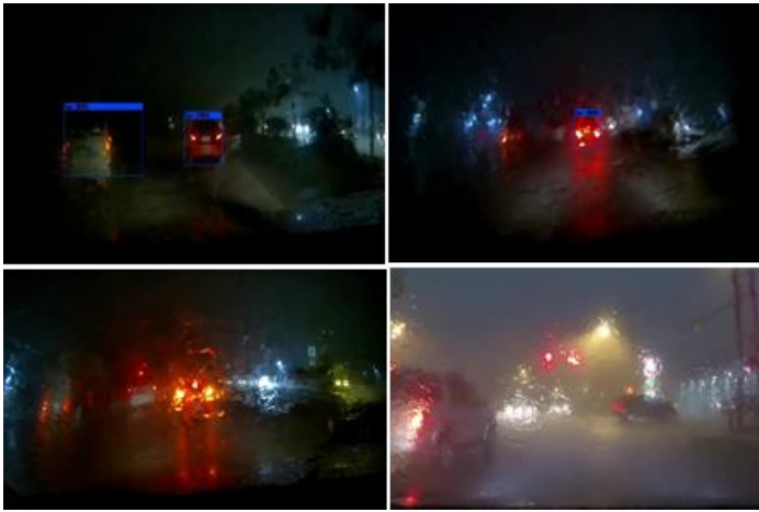
Figure 25. YOLOv3 Detection in Rainy Weather Condition
