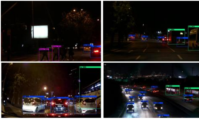
Figure 13. Detection Results for YOLOv4 at Night
