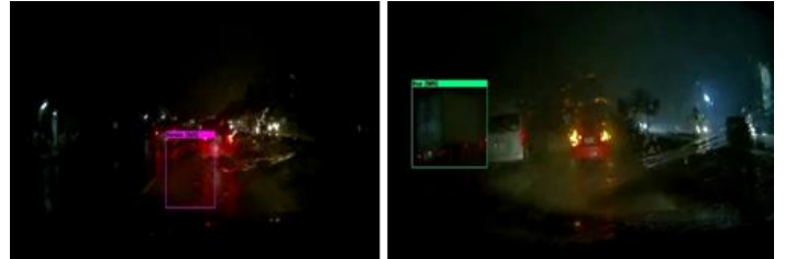
Figure 16. Wrong Detection for YOLOv4 in Heavy Rain at Night
