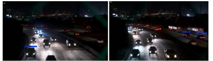
Figure 23. Bad detection of YOLOv3 at Night
