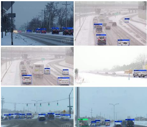
Figure 27. YOLOv3 Detection in Snowy Weather Condition
