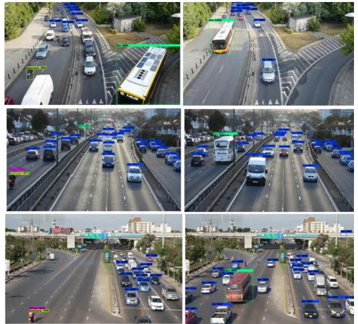
Figure 11. Detection Result for YOLOV4 at Daylight
