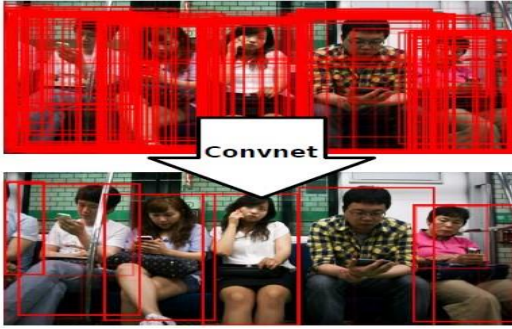
Figure 8. How the Greedy NMS Works (Hosang et al., 2017)
